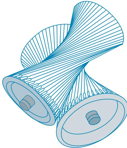
Each of these gears has the shape of a hyperboloid, a type of surface we will study in Section 12.6. The shape allows the gears to transmit motion between skew (neither parallel nor intersecting) axes.
