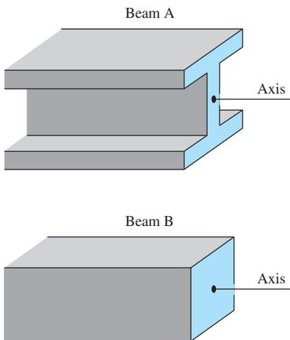
**FIGURE 15.44** The greater the polar moment of inertia of the cross-section of a beam about the beam’s longitudinal axis, the stiffer the beam. Beams A and B have the same cross-sectional area, but A is stiffer.
