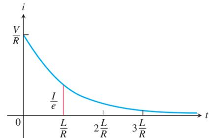
27. **Time constants** Engineers call the number  $L/R$  the *time constant* of the  $RL$  circuit in Figure 9.10. The significance of the time constant is that the current will reach 95% of its final value within 3 time constants of the time the switch is closed (Figure 9.10). Thus, the time constant gives a built-in measure of how rapidly an individual circuit will reach equilibrium.
