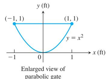
46. The end plates of the trough shown here were designed to withstand a fluid force of 6667 lb. How many cubic feet of water can the tank hold without exceeding this limitation? Round down to the nearest cubic foot. What is the value of  $h$ ?
