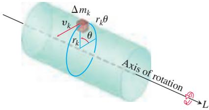
**FIGURE 15.40** To find an integral for the amount of energy stored in a rotating shaft, we first imagine the shaft to be partitioned into small blocks. Each block has its own kinetic energy. We add the contributions of the individual blocks to find the kinetic energy of the shaft.
