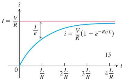
**FIGURE 9.10** The growth of the current in the  $RL$  circuit in Example 4.  $I$  is the current's steady-state value. The number  $t = L/R$  is the time constant of the circuit. The current gets to within 5% of its steady-state value in 3 time constants (Exercise 27).
