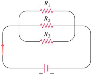
**FIGURE 14.20** Resistors arranged this way are said to be connected in parallel (Example 7). Each resistor lets a portion of the current through. Their equivalent resistance  $R$  is calculated with the formula
